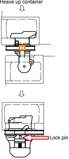
Pushing lock pin to left, turn twist lock clockwise.
