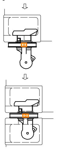
After stack container twist lock is locked automatically.
