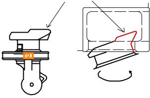
Insert upper fixed cone projecting into corner fitting and turn to counterclockwise. And then twist lock is automatically locked by locking mechanism.
